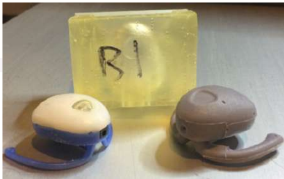
Naked beta 1 prototype, beta 1 prototype with silicone, and beta 1 SLA mold for silicone
